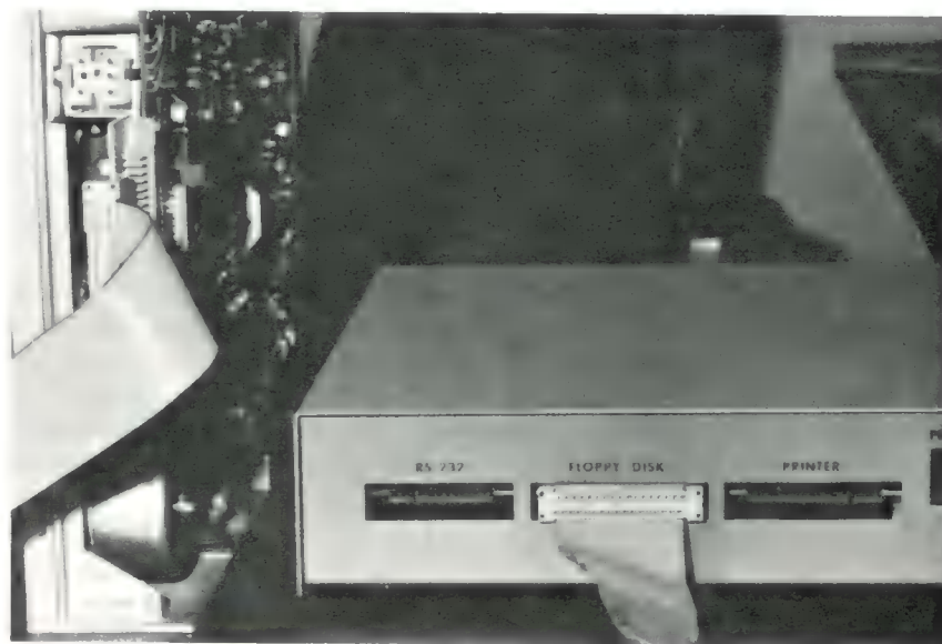
PHOTO #6: Connecting the Standard Drive Cable to the ATR8000
